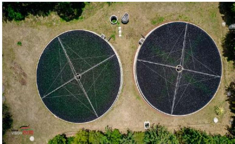
TOP: The aerial view of the water filtration process in the Highrate trickling filters.
